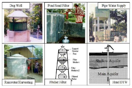
Figure 5.2: Different options of alternate safe water supply in arsenic-prone areas
