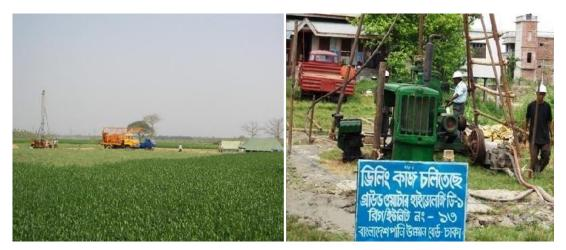
Figure 6.5: Groundwater survey and investigation activities i.e. exploratory drilling by BWDB in the field
