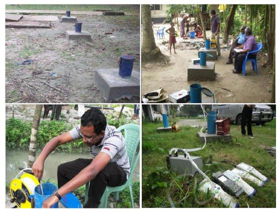
Figure 6.8: Measurement of groundwater table and physic-chemical parameters in the field
