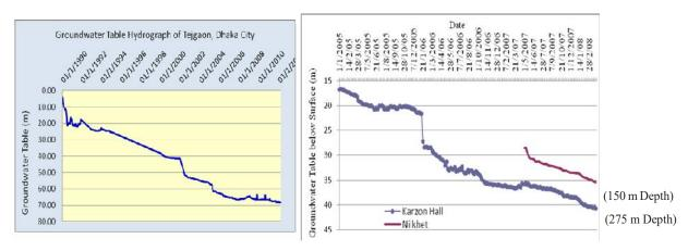
Figure 5.9: Continuous declining trend of groundwater table both in upper and deeper aquifers in Dhaka city
