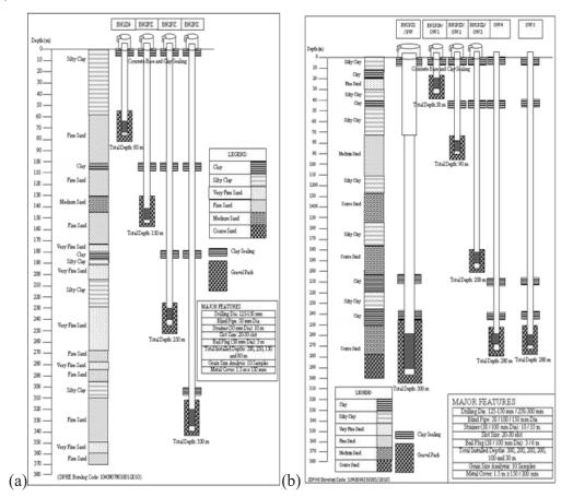
Figure 6.7: (a) Design of installed observation well nest and (b) deep aquifer pump test set-up at Barguna. Both are designed considering borehole lithology and water quality
