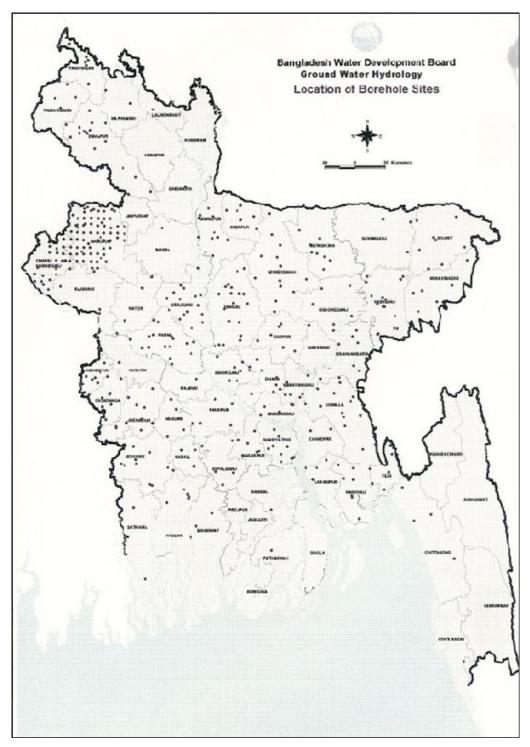
Figure 6.3: Location of BWDB exploratory drilling sites, drilled down to the maximum depths of 350 m
