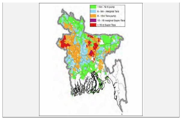
Figure 3.2: Lowest water levels depths measured in 2009 by DPHE
