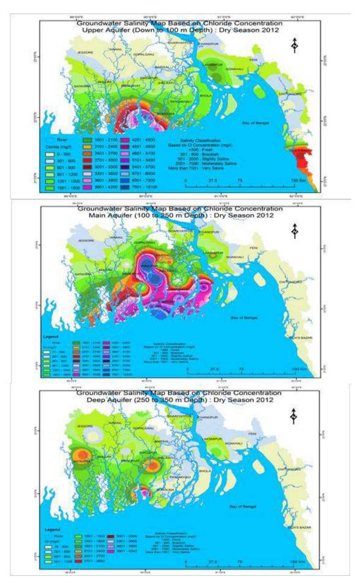
Figure 5.4: Distribution of dry season groundwater chloride concentrations at different depth levels in the coastal aquifers of the Bengal delta (Zahid et. al. 2013)
