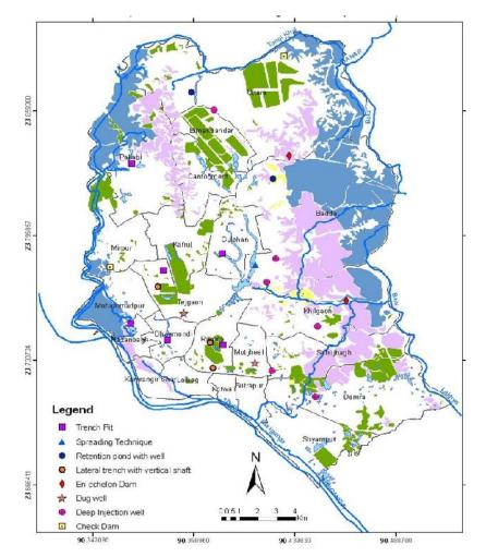
Figure 5.10: Proposed artificial recharge technologies for Dhaka city mainly based on geomorphology and lithologic conditions (Sultana 2009)
