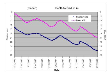
Figure 6.3: Hydrograph of shallow and deep monitoring well at Diabari, Well ID: DMW-2
