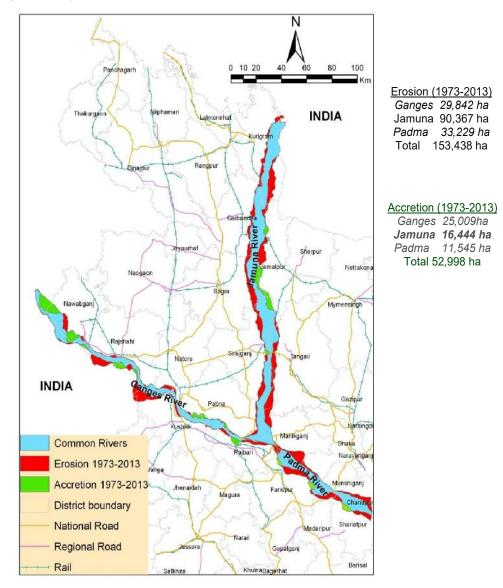
Figure 2.1: Erosion and accretion along the banks of the Jamuna, Ganges and the Padma rivers from 1973-2013
