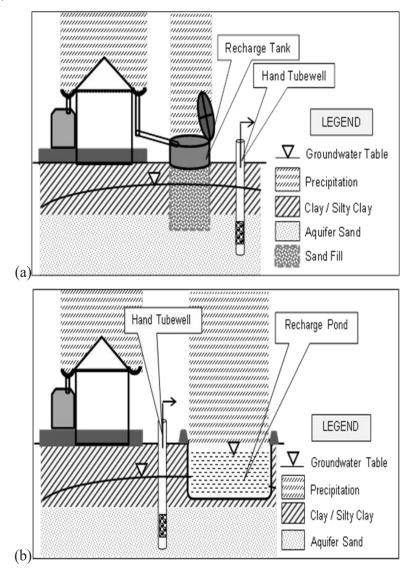
Figure 7.2: Proposed design of (a) Recharge Tank and (b) Recharge Pond to increase fresh water discharge of very shallow wells (up to 5-8 m) in the arsenic and salinity affected coastal areas
