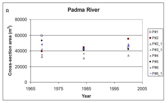
Figure 4.4: Temporal variation of flow area below bankfull stages determined by the analysis of timeseries Standard Cross-sections of the Jamuna and the Padma Rivers surveyed by BWDB
