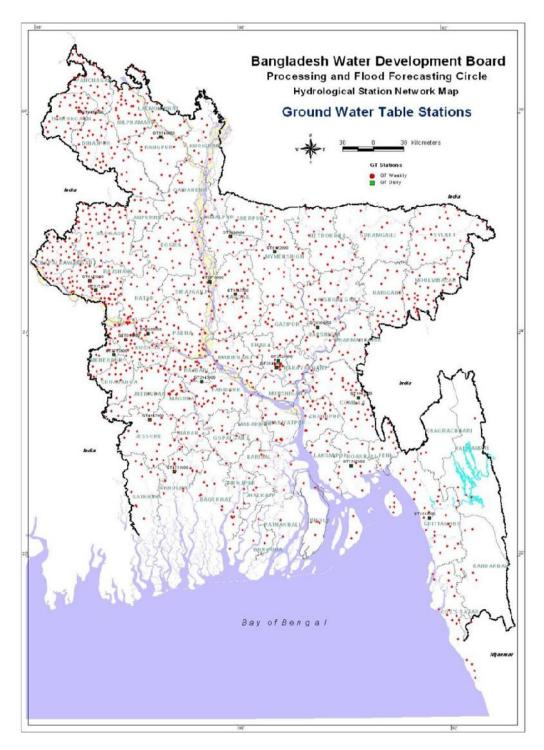
Figure 6.2: Location of BWDB groundwater table monitoring wells installed at shallow depths
