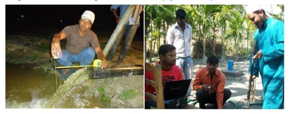
Figure 6.9: Performance of aquifer pump test (a) and slug test (b) in the field to determine the hydraulic properties of aquifer sediment
