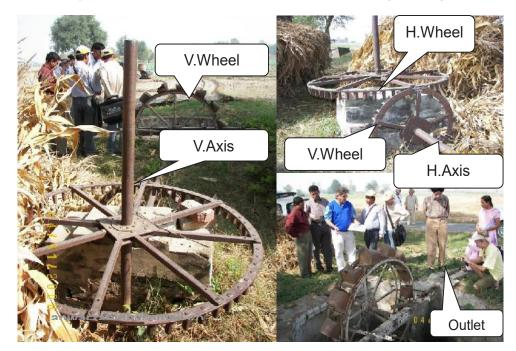
Figure 4.1: Remnants of the previous traditional means of irrigation technology i.e. Persian Wheels in the Indian Sub-continent
